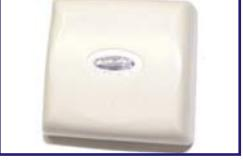
Repeaters automatically form the backbone mesh radio network, relaying messages to/from the Hub. The network physical layout is determined by the placing of Repeaters, which may extend across floors and buildings. Repeaters are battery powered and do not need any wires, making installation very quick and low cost. Each Repeater provides a location beacon signal for accurate location determination for alarm signals and also for tracking.
