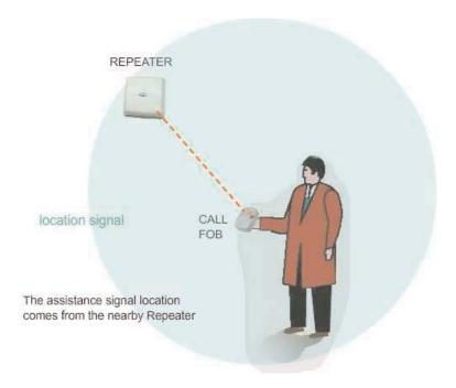
When a user signals an alarm, the user identification (name), location and alarm type are included in the alarm message displayed on the Hub and sent to Pagers.
